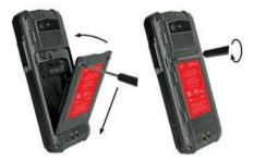
» Place the battery in the battery compartment as shown.
