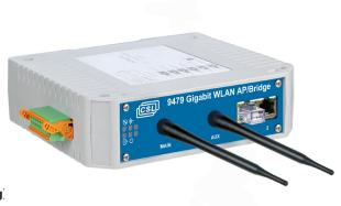
The 9479-ET-CSL is an Intrinsically Safe (IS) WLAN AP/Bridge Module suitable for Zone 1 / Zone 21 mounting, (Zone 0 / Zone 20 with a suitable Ex ia Power Supply).
