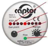
LED chain for display of flow speed
