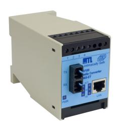
The 9465-ET 10/100Mbps Copper to Fibre Optic Media Converter allows an Ethernet network to be extended over a greater distance. A multi-mode fibre optic link may be up to 2km in length when running at 100Mbps and due to the use of 1300nm optics an extended distance of 5km is achievable at 10Mbps. Longer distances are achievable with single mode fibre.
