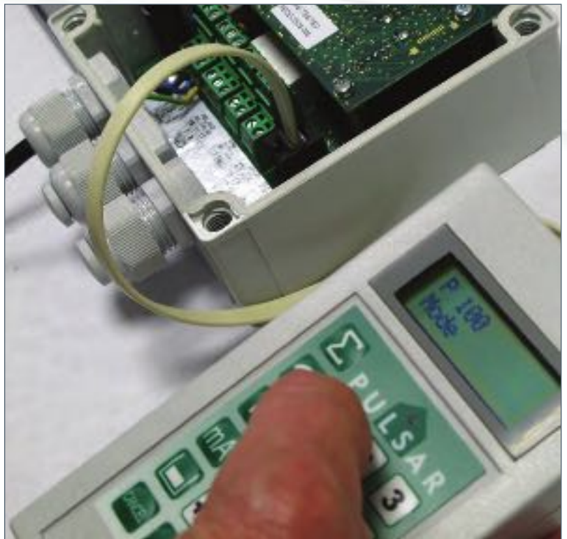
REMOVABLE HAND-HELD PROGRAMMING UNIT CONNECTED TO BLACKBOX
