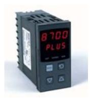
The West 8700+ is a programmable safety cut out with optional outputs for annunciators and alarms. A latched relay cuts power to your process if safe values are exceeded. The unit must be reset before the process can continue. It has the improved Plus Series hardware and user interface for optimal ease of use.
