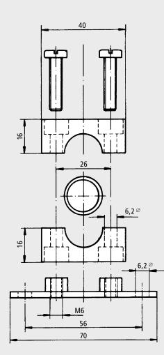
Width of the welding plates:30 mmThickness of the welding plates:7 mm
