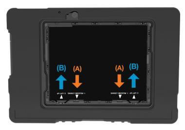
Release locking by pulling on the battery holder hook (A) towards the bottom of the device then pull the battery up (B). Repeat process for other battery holder hook.
