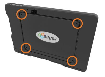
Remove the 4 screws from the corners of the battery cover using the provided tool. 2. Take off the battery cover by pulling on the cover carefully - specifically on the corner with the slant.
