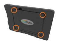
Then replace the 4 corner screws of the battery cover using the provided tool. The recommended torque for the screw is 10-12 Ncm.
