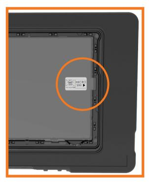
4. Enter the Micro SIM card into the slot in the center of the right side. Make sure you have the Micro SIM card in the correct direction (chip facing down). Attention! Only Micro SIM card to be used. Do not use Nano-to Micro SIM card adapters!
